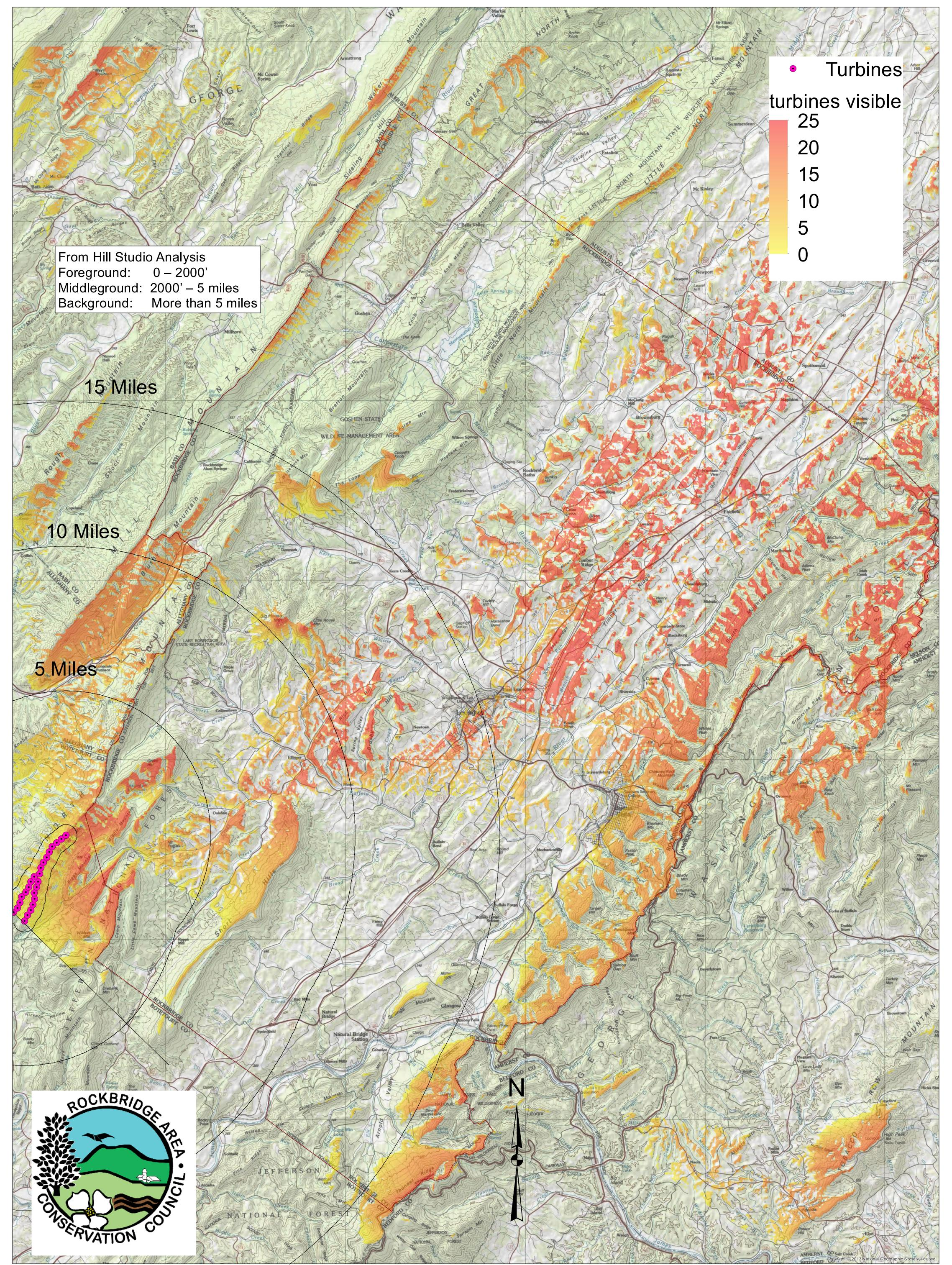
Wind analysis conducted in ArcGIS10.3 using USGS NED 30 m elevation data and bare earth assumption. Model tower/blade height is 550 ft with locations estimated from application documents. Limited to arc from north (0) to SE (145 degrees) and to NAD\_1983\_UTM\_Zone\_17N Prepared by David Harbor January 21, 2016
